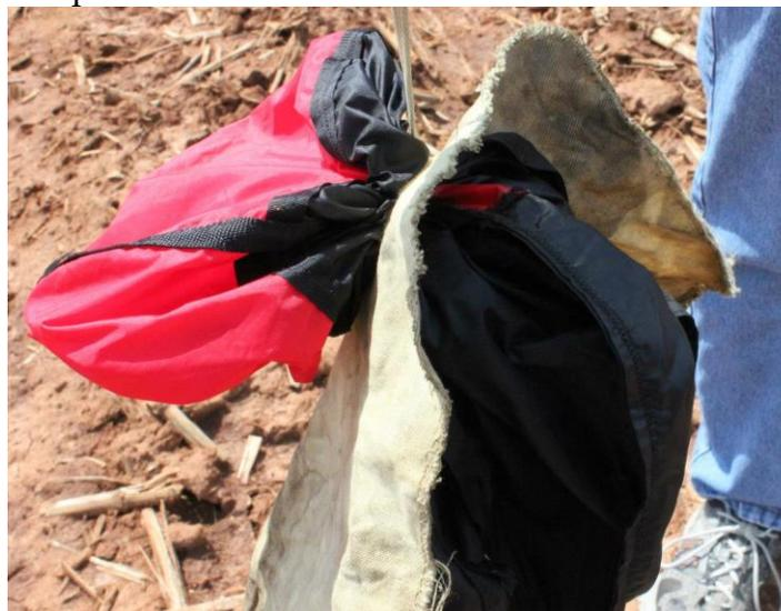
Figure II-2 Drogue chute partial failure
