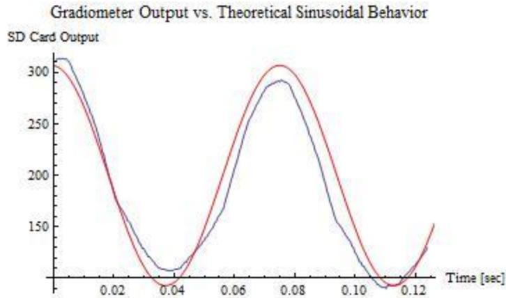
Figure III-1 Theoretical Behavior at 6.6 Hz (Red) vs. Measured Result (Blue)
