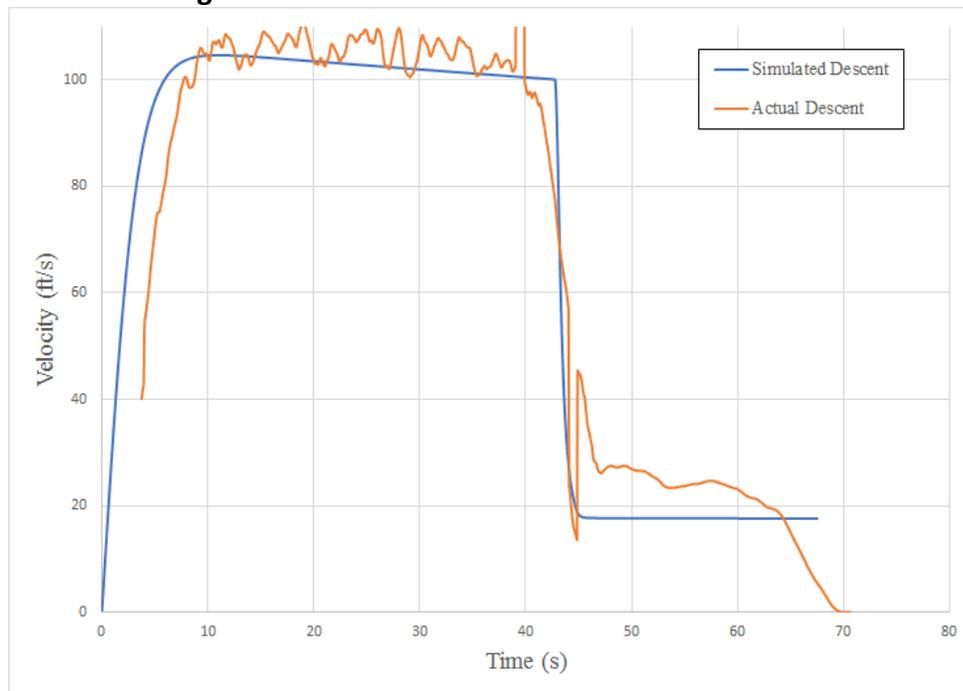
**Figure 3: Velocity v. Time of Rocket During Descent**
