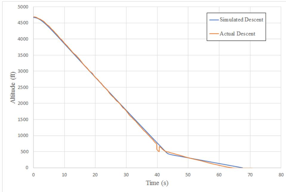
**Figure 2: Altitude v. Time of descent of rocket**
